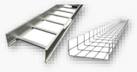
80% of industrial applications. Ladder-type cable trays effectively prevent moisture accumulation, making them ideal for general use. For sensitive circuits, we recommend solid bottom cable trays, which provide superior EMI/RFI protection due to their solid bottom and cover.
